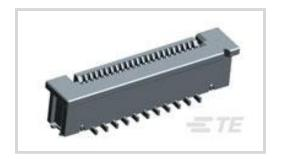
Connector System: Flex-to-Board Number of Positions: 8 Centerline (Pitch): .5 mm [ .02 in ] Insertion Force Type: Zero Insertion Force (ZIF) PCB Mount Orientation: Vertical
